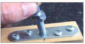
Raise the door and screw the roller bolt into the mounting plate on the top of the sliding door. →
