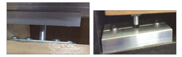
**12.** Adjust the level of the door by screwing in or out the pivot at the bottom of the pivoting door and the roller bolt at the top of the sliding door. The door is properly adjusted when the door moves smoothly with the roller.
